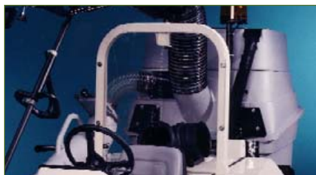
A unique, sturdy rollover protection system (ROPS) safeguards operators.
