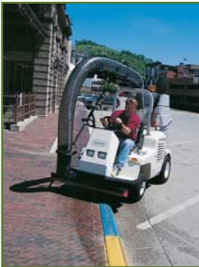
A four-wheel stance provides greater stability, lessens the risk of tip-overs, and gives a smooth ride.
